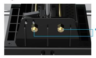
Tighten the screws and fix it with nuts.
